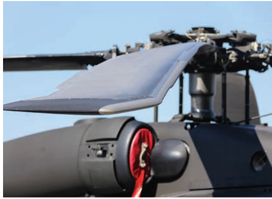
Leading edge abrasion strips for rotorcraft blades are manufactured by AlphaCoin. (Photo courtesy AlphaCoin)
